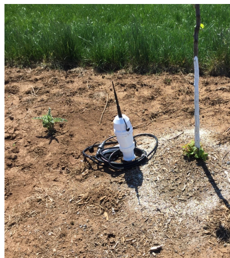
Figure 3: Soil Moisture Sensor system in hops
