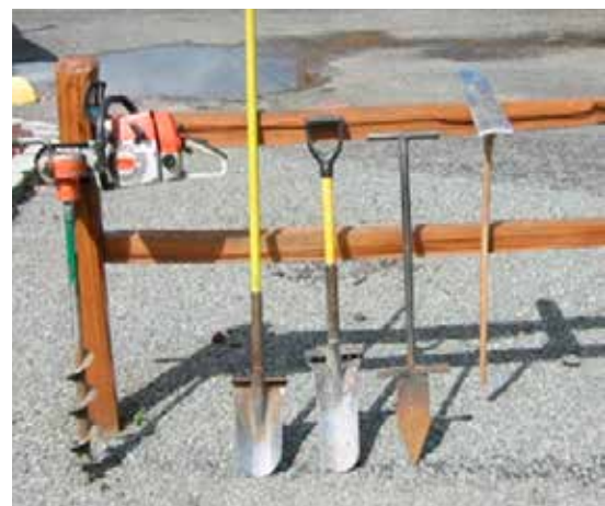
Specialized tree-planting tools, from left: power-driven auger, long-handled and short-handled planting spade, dibble bar, and hoedad.
