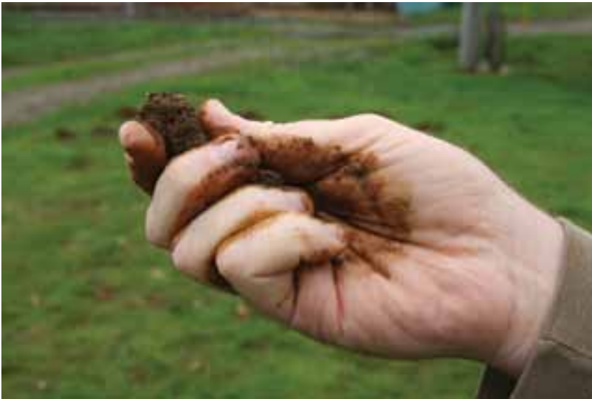
Figure 7b: Using a soil ribbon to test soil for clay, loam, or sand content. The longer and firmer the ribbon, the more clay content in the soil. (Photo: Gina Emanuel)
